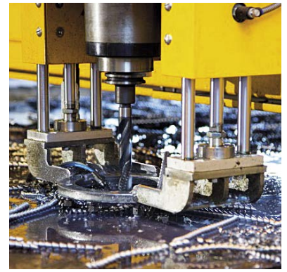
Drilling and tapping heads with automatic tool exchange and measurement of drill lengths; cleaning chips off plates after drilling
