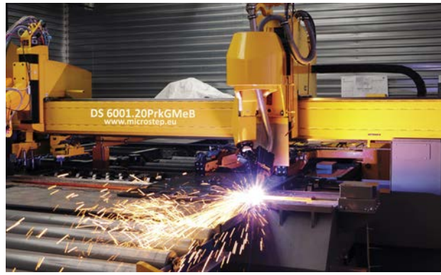
5-axis plasma head with infinite rotation enables bevel cutting of sheets with a tilt of up to 50°; ACTG increases accuracy of bevel cutting with a plasma rotator
